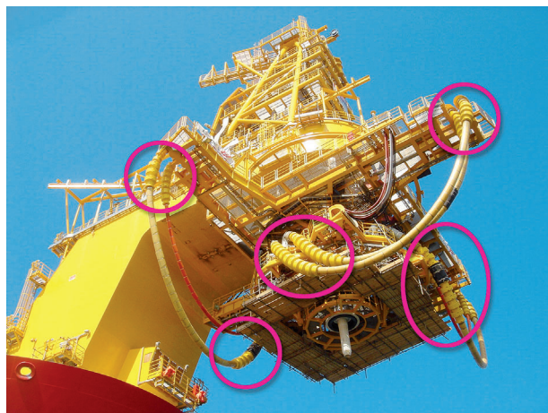
Figure 15. Loading tubes with cable and bend restrictor elements (circled) made of PU elastomers on an offshore loading crane.
